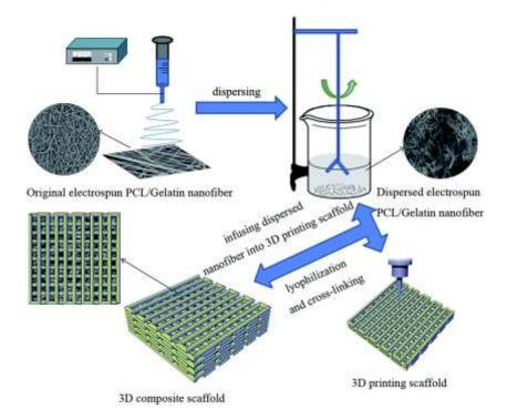
Figure (3) Fabrication and characterization of electrospinning/3D printing bone tissue engineering scaffold
